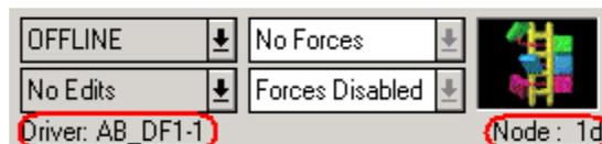
19) Use the off line pull down tab to download to the processor.
