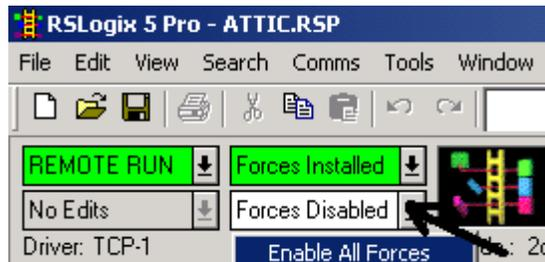
The force light on your processor will now be solid amber indicating that installed forces have been enabled. If we go to the data table, you will see that the input bit is on, and it is red indicating that a force has been enabled on the input.
