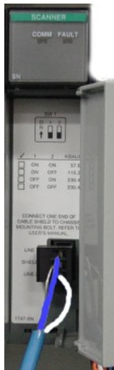
The dip switches must be configured on the 1747-SN module for the correct baud rate. Baud is a term to describe how many bits per second are transferred over the network. Below is a photo of the switches. You will find a sticker inside the door of the scanner displaying the correct switch configuration for each available baud rate.
