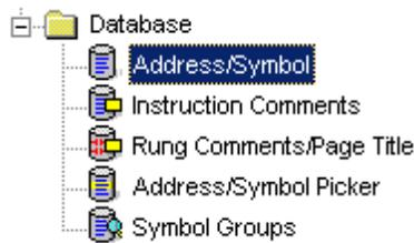
6) When entering a symbol in logic, the symbol actually goes into the documentation database. Open the Address/Symbol editor, and locate the symbols we typed in the ladder view.
